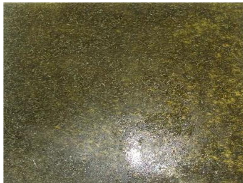
Fig.3.2-Pine needle short fiber reinforced composites
