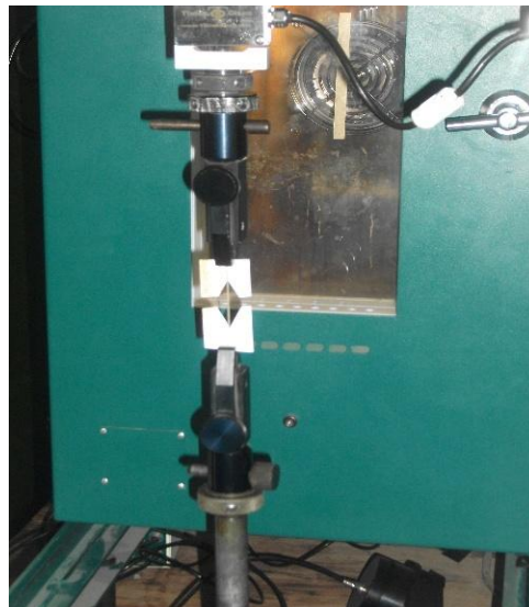
Fig.2.2- Specimen clamped on machine
