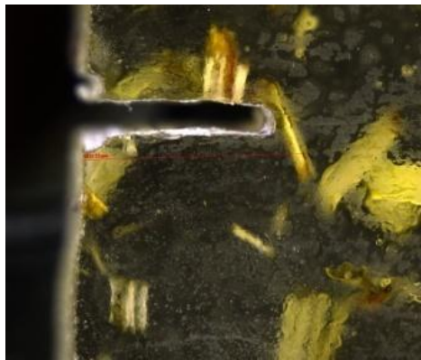
Fig.3.5- Stereo-microscopic image of the crack along with notch
