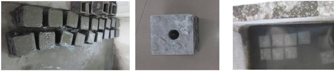
Fig 3 Casting and Curing of Specimens
