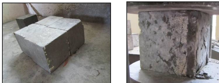
Fig 8 Whitish Appearance on Specimens after Sulphuric Acid Curing
