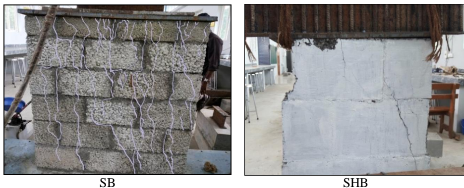
Fig 14 Failure Pattern of SB and SHB
