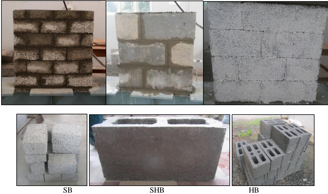
Fig 9 Masonry Wall Built using SB, SHB and HB
