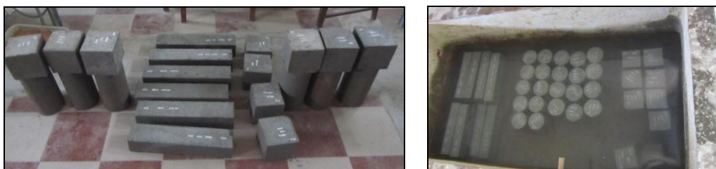
Fig 5 Casting and Curing of Specimens
