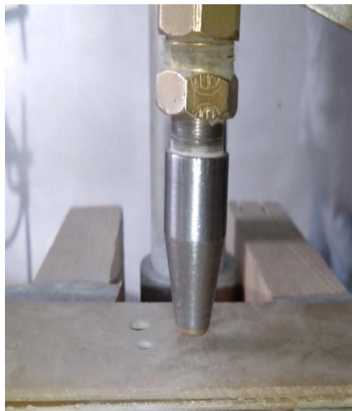
Fig 2: Impingement of Abrasives through Nozzle
