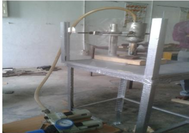
Figure 8: Abrasive Jet Machining Setup established at SMEC
