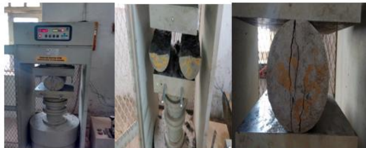
Testing of the cylinders for the Split Tensile Test
