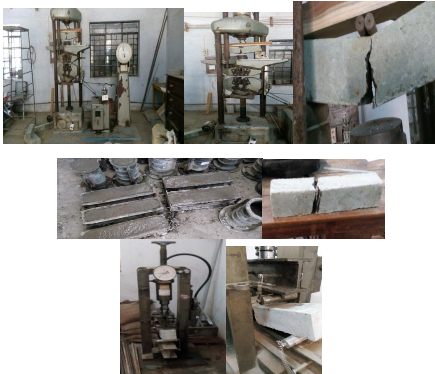
Testing of Beams for Flexural strength test
