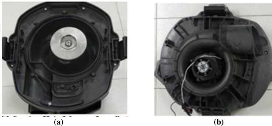
Fig. 3 (a) C5: Suction unit (Motor + Impeller), (b) C6: Suction unit with only motor
