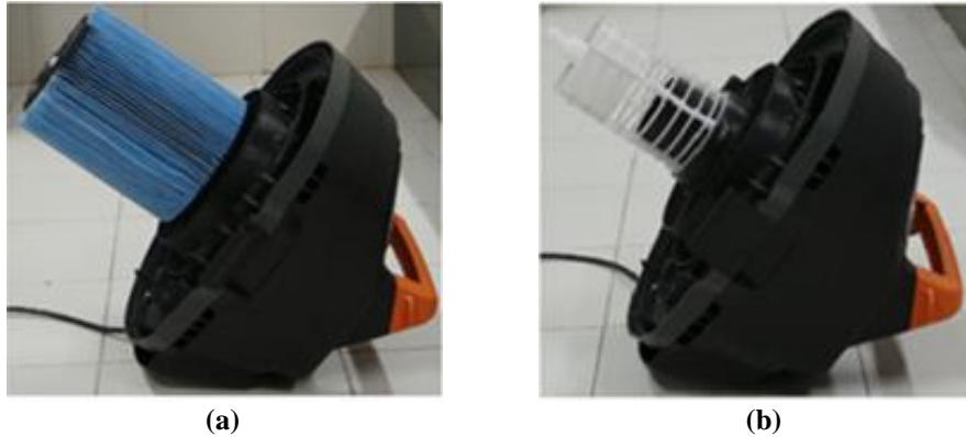
Fig. 2 (a) C3: Vacuum cleaner without drum with filter, (b) C4: Vacuum suction unit without drum and filter
