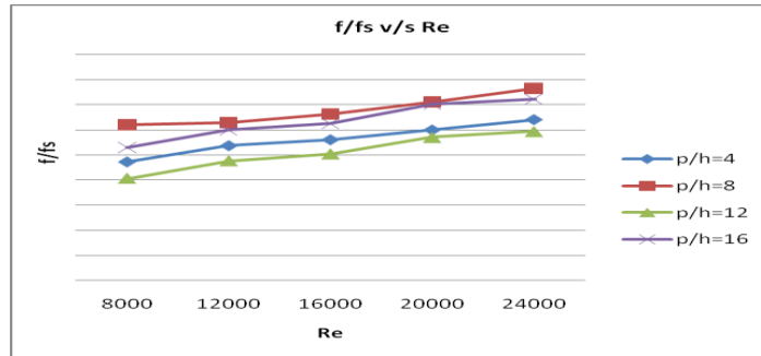
Fig 3. Variation of f/fs with Re ( AR=5 , h=6mm , Perforated ribs with 2mm dia. holes)
