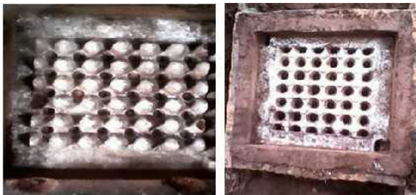
Plate 4.2: Left: Finished sand mould (Drag); RIGHT, finished sand mould (Cope)
