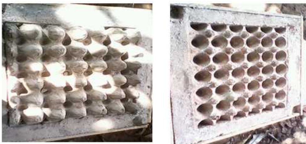
Plate 4.1: Left; cope pattern, Right; drag pattern
