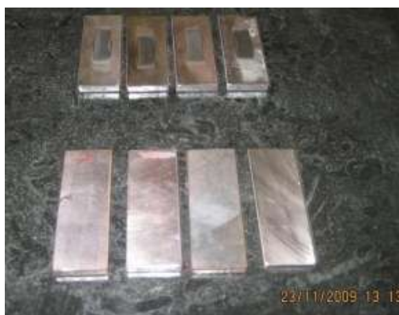
Figure 1. Standard Test Specimen Of Size 75mmx 26mmx6mm
