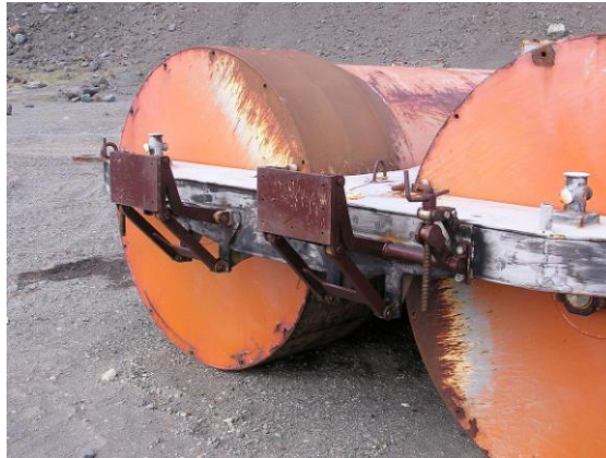
Fig. 4. The proposed device may form a ‘barge’ once fitted with an outboard motor. The example shown here has been used at the Henryk Arctowski Antarctic station in the South Shetland Islands.
