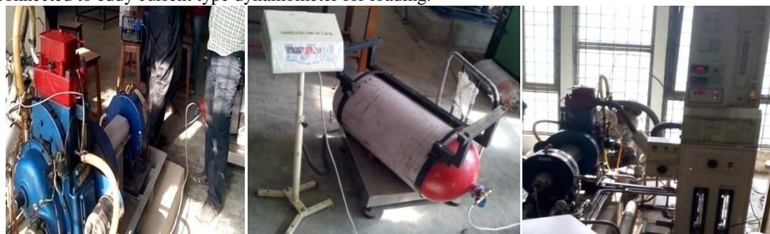
Fig. 1: Actual Photo of experimental setup showing engine, cylinder, weighing scale
