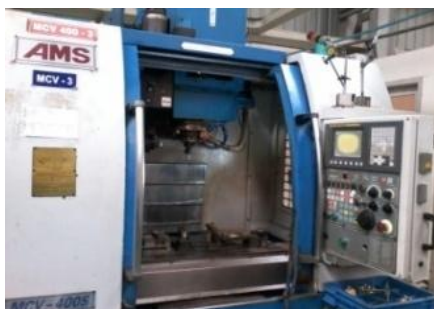
Figure 1 Vertical machining centre MCV 400S
