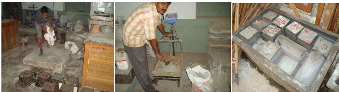
Figure 2.2 Shows Mixing of materials, weighing of materials and curing of concrete.
