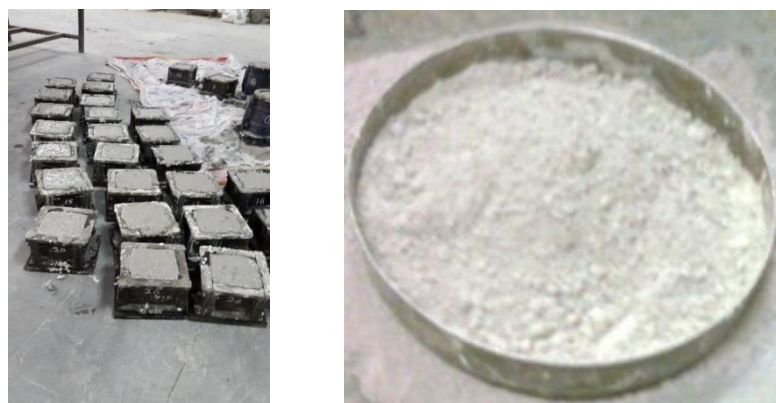
Fig. 1 Shows Cubes after Casting Fig.2 Shows Ground Granulated Blast Furnace Slag (GGBS)
