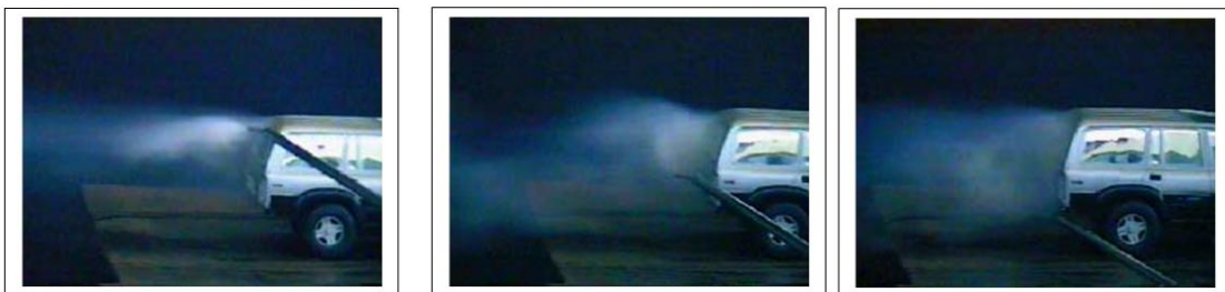
Figure (9): Re-circulating bubble or spiral vortices at the rear part of TOYOTA model
