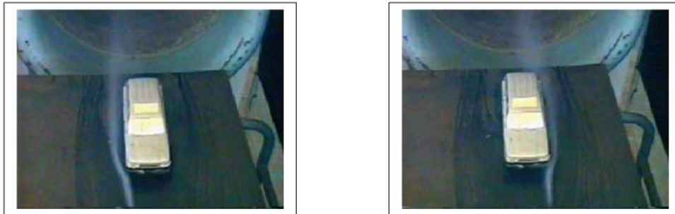
Figure (8): Attached flow at the right and left sides for TOYOTA model
