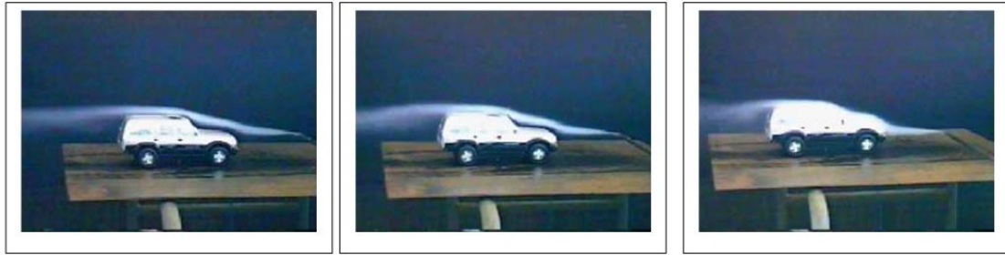
Figure (7): Flow visualization around TOYOTA model
