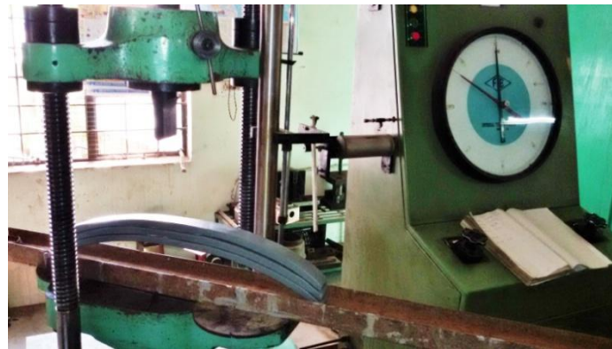
Fig. 16: Testing of SFRC Leaf Spring
