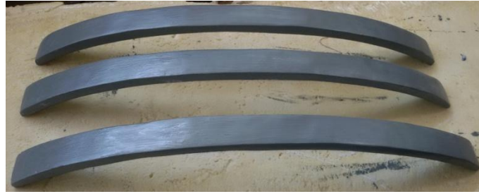
Fig. 15: SFR Composite Leaf Spring after coating
