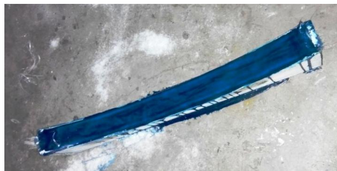
Fig. 14: Raw leaf spring after curing
