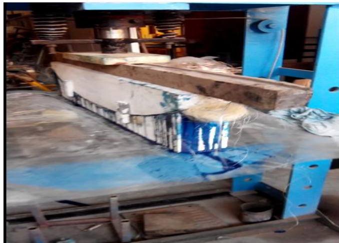
Fig. 13: Light compression moulding of composite Leaf Spring.
