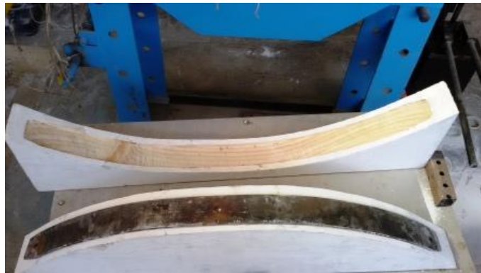
Fig. 12: Wooden mould for Leaf Spring
