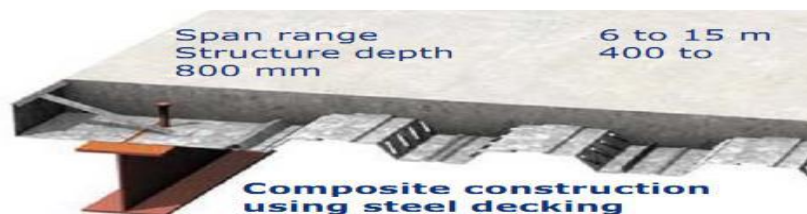
Fig. 2. Typical Composite Slab
