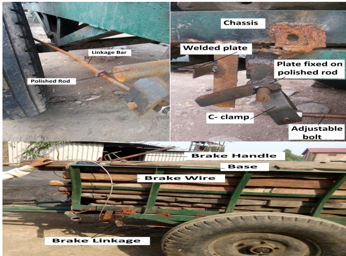
Fig. 3.4: Implementation of braking system on cart
