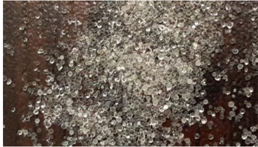
Fig.1: Glass beads used as a fine aggregate
