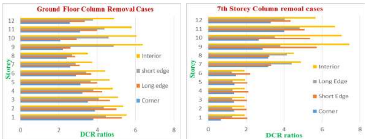
Fig 6 DCR ratio of beams for flexure for all column removal cases at GF and 7th storey
