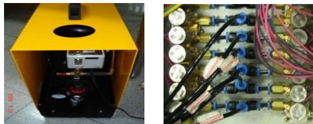
Fig. 2 Air pressure system a) Air compressor, b) Solenoid valves and air hoses [17]
