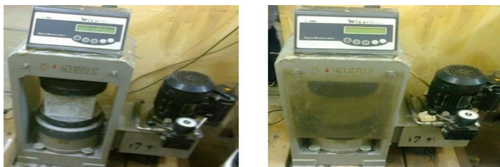
Figure 6: Cube Specimen under Compressive Loading
