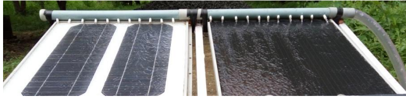
Fig.3. Close-up of the flowing film of water at the PV module surface
