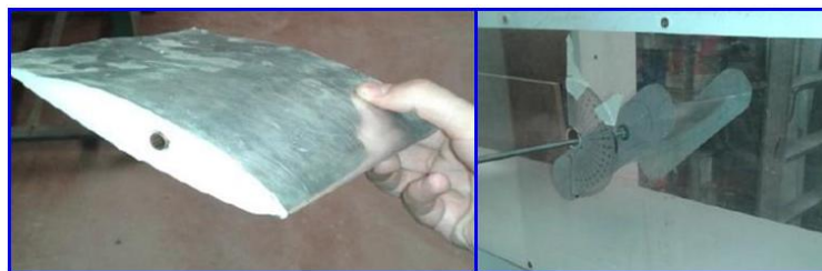
Figure 7: small wing built on an airfoil S813, and wind tunnel testing.
