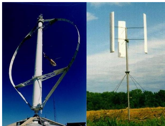
Figure 1: (a) Conventional Darrieus - (b) Darrieus-H or Giromill.
