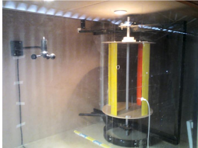
Figure 10: Model Darrieus turbine-H tested in the wind tunnel No. 2 of the FI-UNCo.
