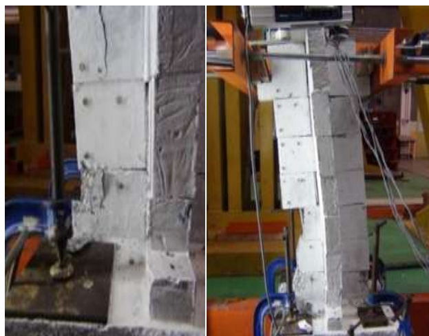
(a) Crushing at 3rd Block. (b) Crushed 4th and Last Block
