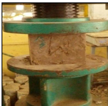
Figure 16: Compression test of Geopolymer concrete
