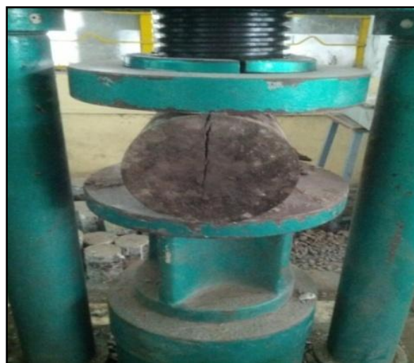
Figure 18: Split Tensile Test of Geopolymer concrete
