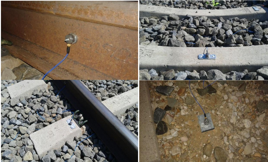
Fig.3. Position of the accelerometers in the different monitored track elements
