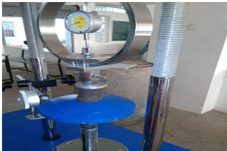
Fig 4.3 Unconfined Compression Strength Test
