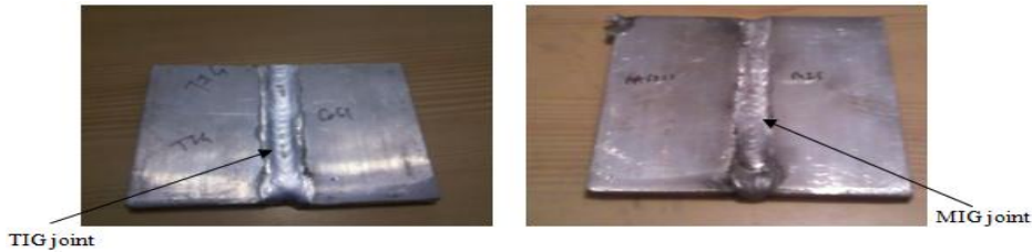
Fig. 5: Actual representation of TIG and MIG weld joint
