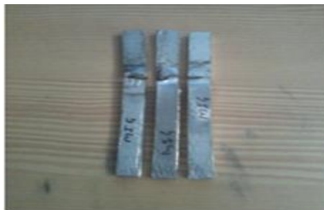
Fig. 6: MIG weld specimen after Izod test
