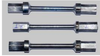
Figure 8: Ready-to-test welded specimens.
