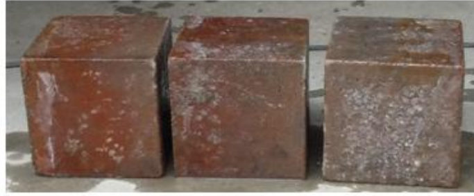
Fig 6 Specimens of Acid Exposure
