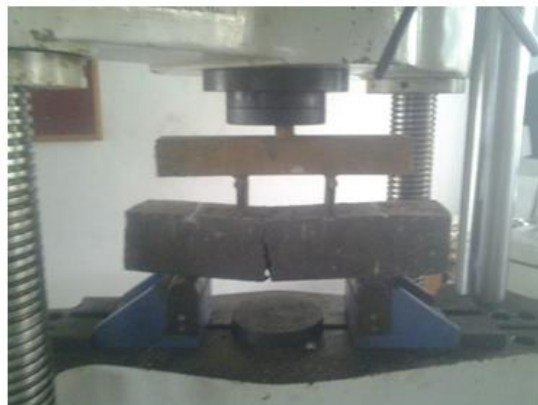
Fig 5 Testing of Prism Specimens
