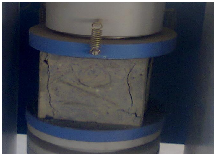
Fig.3 Testing of Cube Specimens
