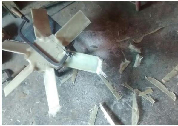
Fig.2 Performing trimming operation on the fan
