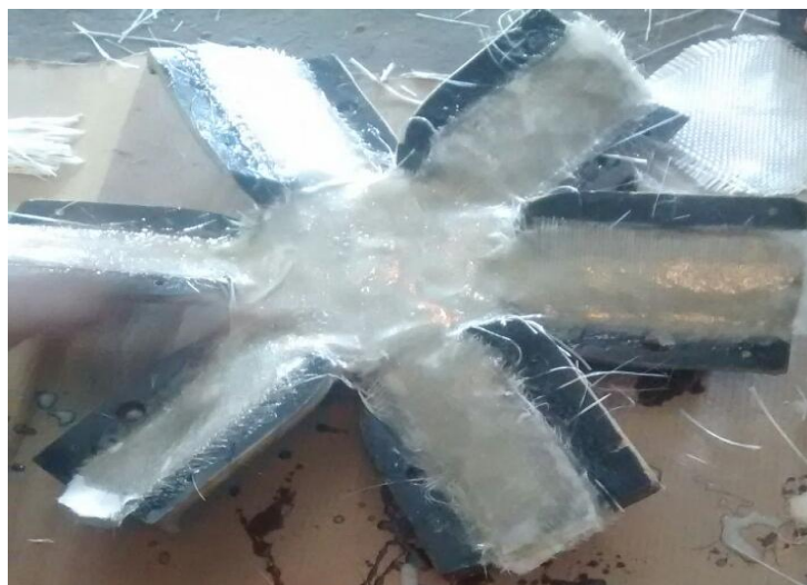
Fig.1 mould used for fabrication of fan with hand lay-up technique
