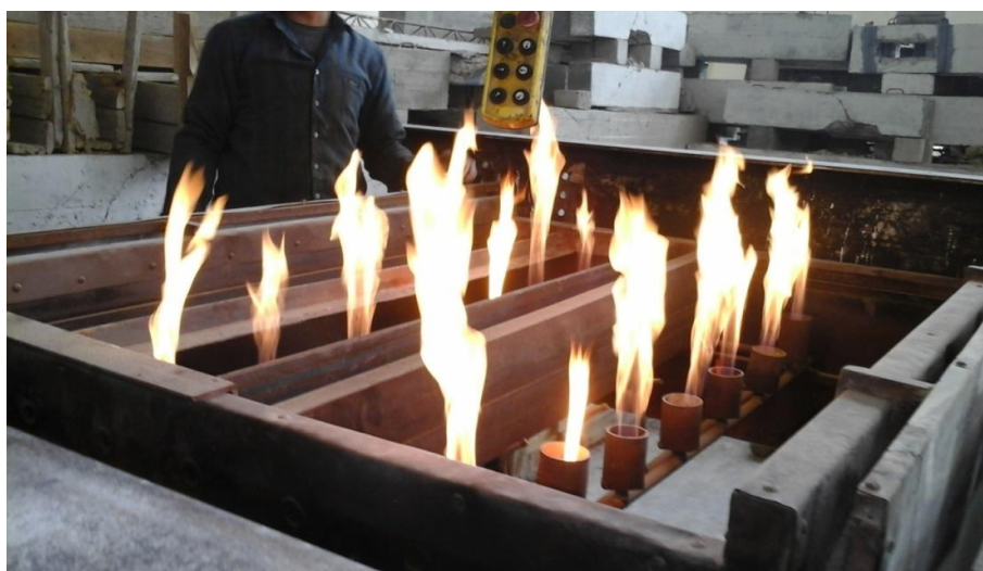
Fig. (9) Multi-burners Furnace with Thermal Insulation.
