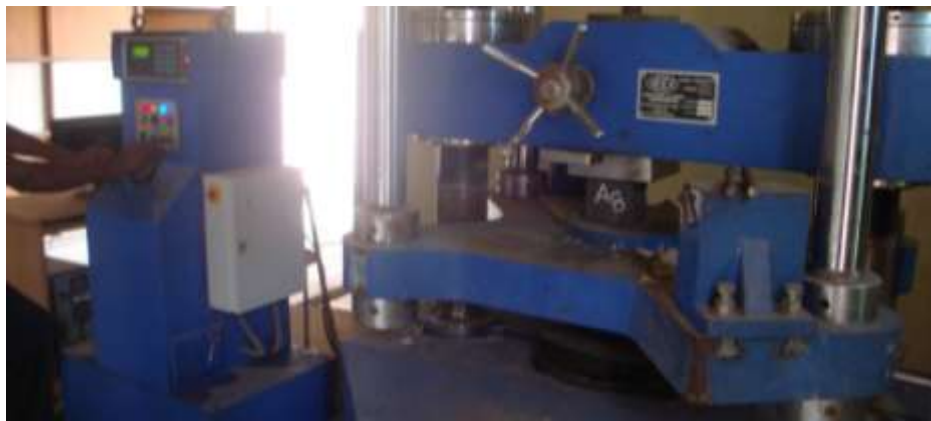
(c) Mortar compressive strength test
