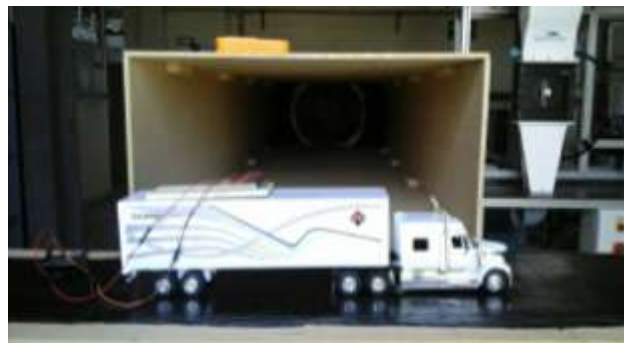
Fig. 4. Experimental phase on the wind tunnel.
