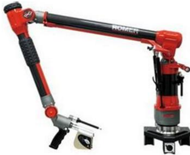
Fig 1. Articulated arm coordinate measuring machine
