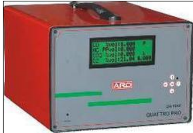
Fig. 7: Exhaust gas analyzer
