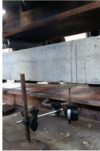
a- Dial gauge is installed to measure deflection.
