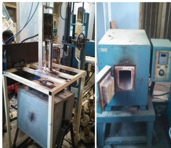
Fig 2 stir casting & preheat setup
