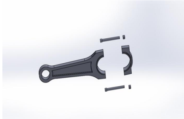
Fig 7 Design of connecting rod
