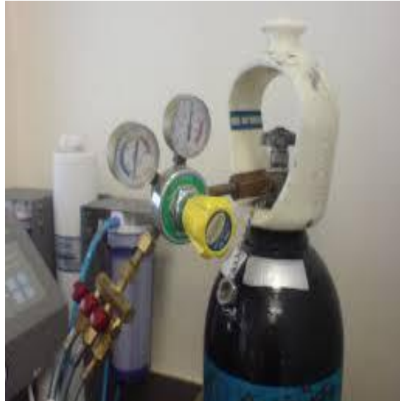
Fig.2.1 Pressure meter with Helium gas cylinder
