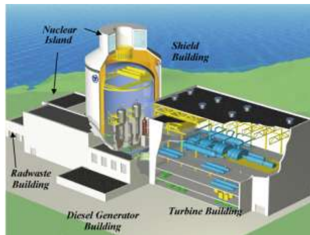
Figure 1: Principle buildings of AP1000 nuclear plant [2]
