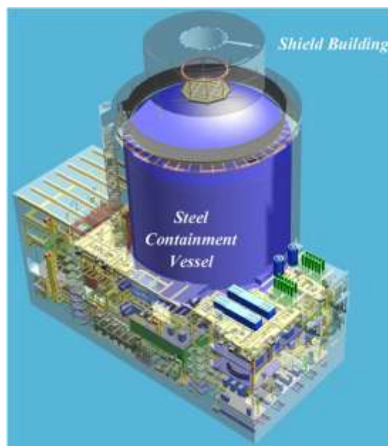
Figure 2: AP1000 nuclear island building [2]
