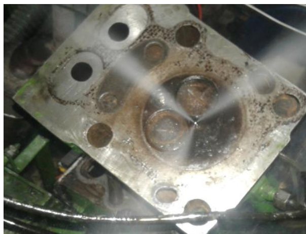
Fig. 1. Spark plug and injector position in cylinder head
