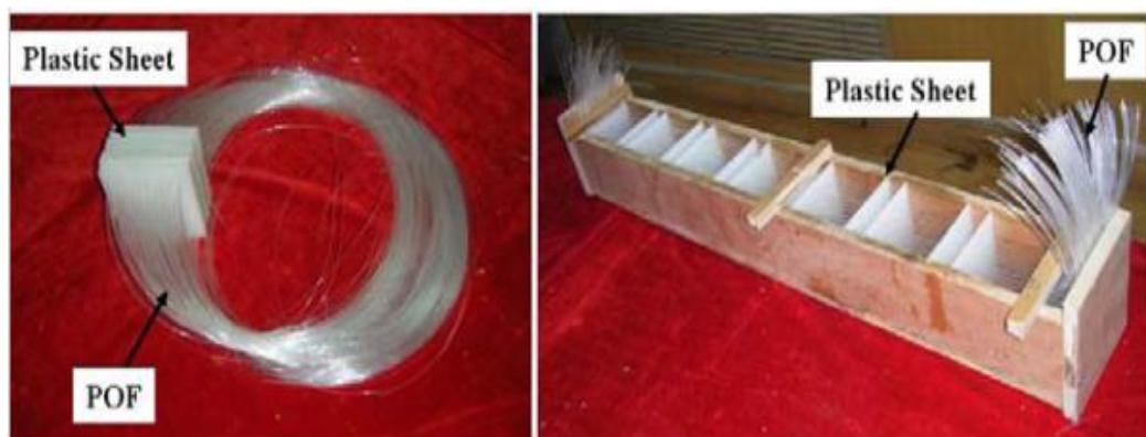
Fig.3.1.1 : Placement of Optical Fibre [7]
