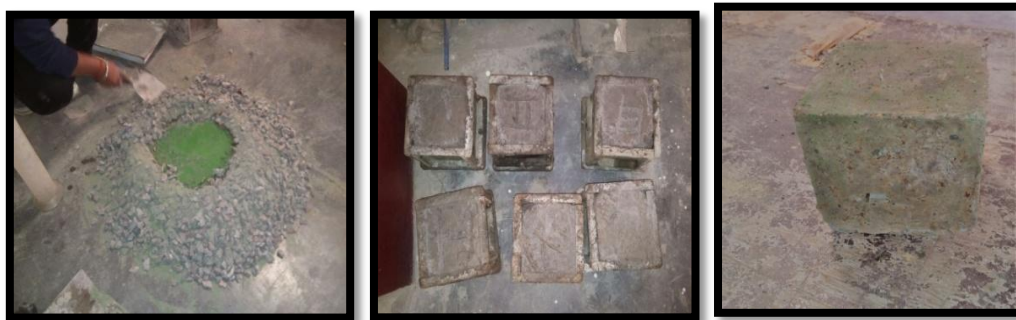
Figure 2: Steps of casting
