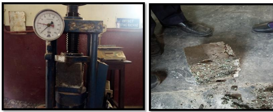
Figure 3: Compressive strength test of sample and cube after failure
