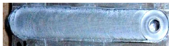
Fig. 3 Typical AA7075/MWCNT Surface composite billet fabricated through FSP
