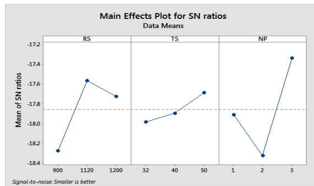
Fig. 5 The Main effects plot for S/N ratios of Wear Rate Vs RS, TS and NP
