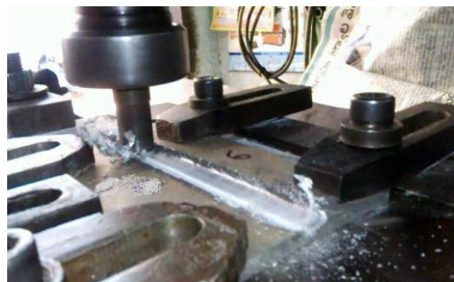
Fig. 2 The FSP carried out on AA7075 billet
