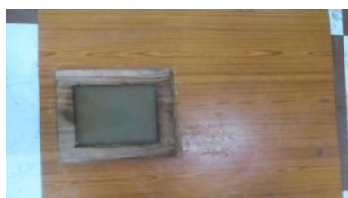
Fig.4. Wooden mould and cast specimen
