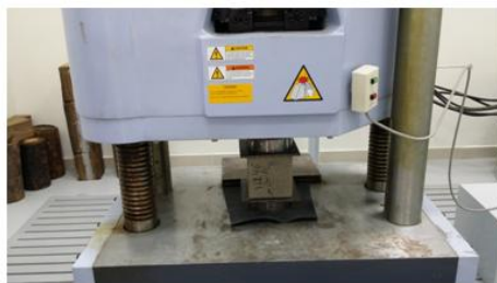
Fig.16 Testing of Cubes
