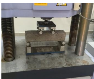
Fig.18 Flexural Strength of Prism
