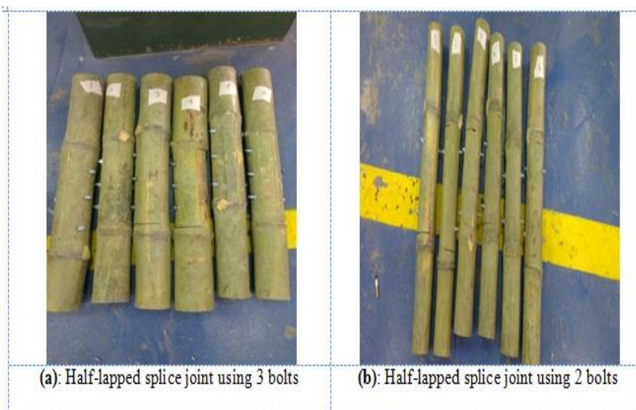
Figure 2: The bolts joint types of bamboo
