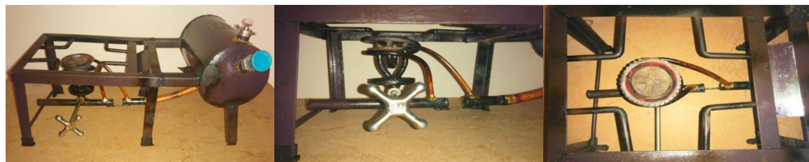
Fig.5: Horizontal Type Pressurized Kerosene Stove
